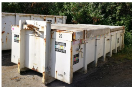
Closed container with sliding roof for gyproc/plasterboard E.g. 10 m 3
